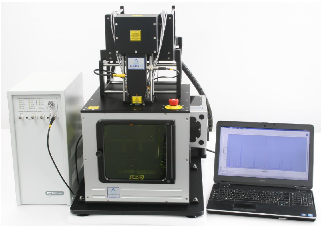
Typical system configuration: LIBS-8 module, Litron Nano SG 150-10 laser head, LPU 350 laser power supply, AP-Nano S adaptor platform (for mounting laser head to LIBS-8 module), XYZ-750 modular sample chamber, SpectroModule-8 eight channel LIBS spectrometer
